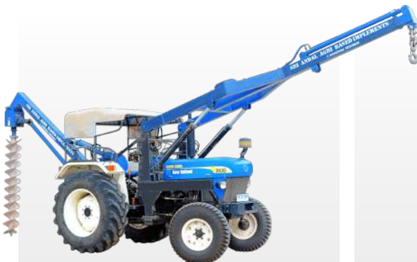
Post Hole Digger with Crane
